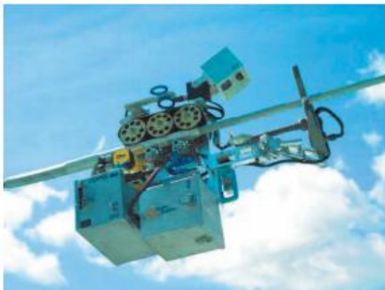
Figure 3.1-11 LineROVer Robot from Hydro-Québec (Photo courtesy of IREQ, © Hydro-Québec)
