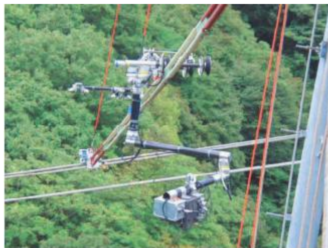
Figure 3.1-4 Expliner Robot from HiBot (Debenest et al. 2010, © 2010 IEEE)
