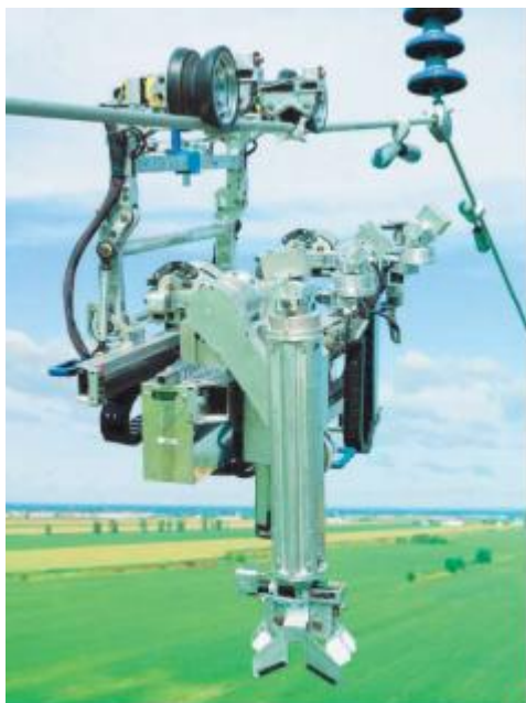
Figure 3.1-1 LineScout Robot from Hydro-Québec
