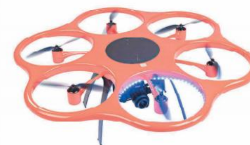
Figure 3.2-9 Example of Hexacopter with Propeller Side Protection and Camera for Visual Inspections (Diameter about 1 meter)
