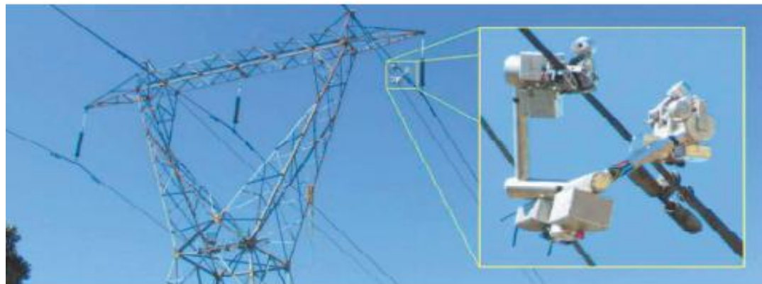
Figure 3.1-7 Power Line Inspection Robot (PLIR) from the University of KwaZulu-Natal
