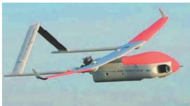
Figure 3.2-2 AAI Aerosonde (Cruise Speed 27 m/s, Payload 8 kg)
